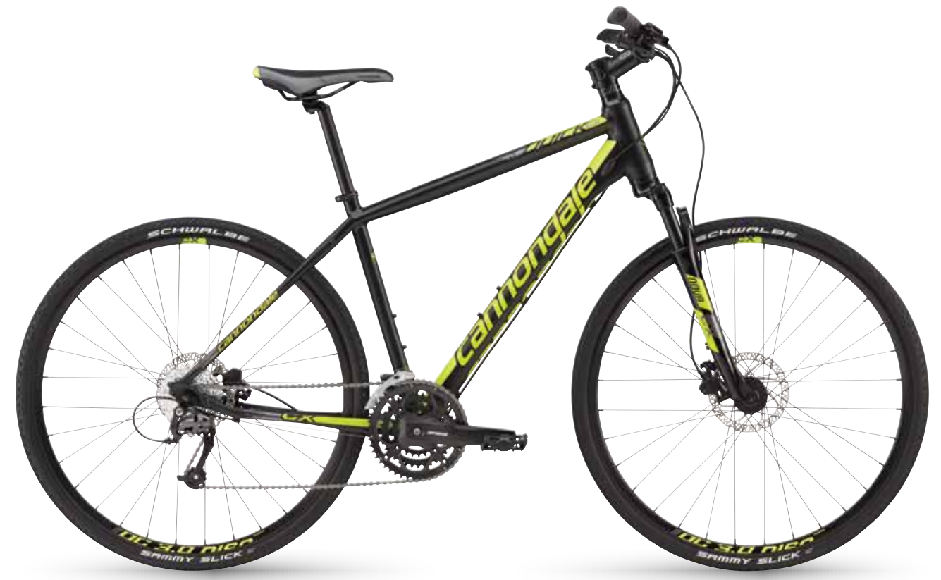
QUICK CX 3 FRAME: Quick CX, Optimized 6061 Alloy FORK: RST Nova 1.5", ML lockout, 50mm RD/FD/SHIFT/CRANK: Shimano Acera/Altus/Altus/FSA Dyno Drive, 48/36/26 BRAKES: Tektro Auriga hydraulic disc WHEELSET: Maddux DC 3.0, double wall/Alloy CX Disc TIRES: Schwalbe Sammy Slick w/Puncture Protection, 700x35c COLOR: Jet Black w/Neon Spring, Charcoal Grey, Matte - BBQ
