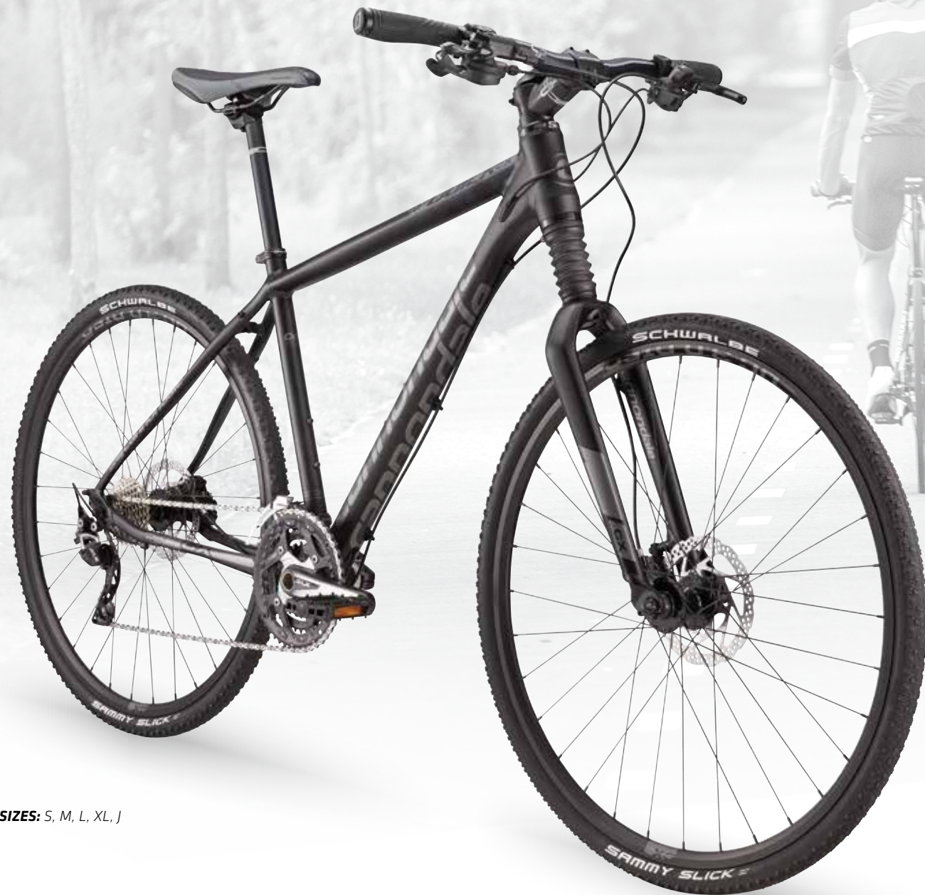
QUICK CX 1 FRAME: Quick CX, Optimized 6061 Alloy FORK: HeadShok Fatty DL50, 50mm, Isolated Damper Technology with lockout RD/FD/SHIFT/CRANK: Shimano SLX/Deore/SLX/SLX, 48/36/26 BRAKES: Shimano M396 hydraulic disc WHEELSET: Maddux DRX 3.0, double wall/Alloy CX Disc TIRES: Schwalbe Sammy Slick w/Puncture Protection, 700x35c COLOR: Jet Black w/Charcoal Grey, Matte - BBQ
