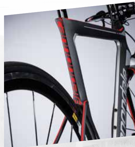
TAP TUBES The TAP (Truncated Aero Profile) tube shapes offer the perfect blend of wind-cheating aerodynamics, efficient stiffness and feathery weight.
